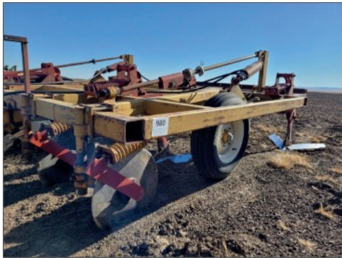
Image 1. Photo of the undercutter sweep used in the trials to conduct mechanical control in early summer.
